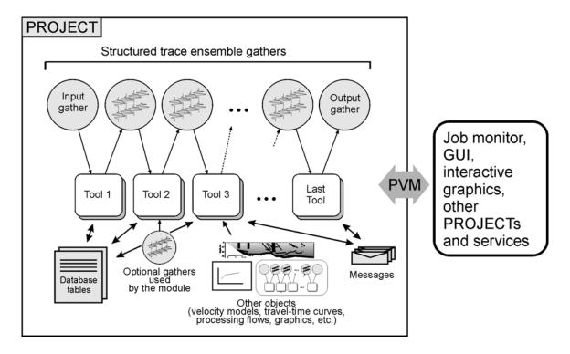
Figure 1. Structure of SIA processing flow, represented by class PROJECT (modified after Morozov and Smithson, 1997). Processing flows consist of linked sequences of tools sharing structured trace ensemble gathers (normally corresponding to multicomponent seismic records), database tables, and various custom data objects.
